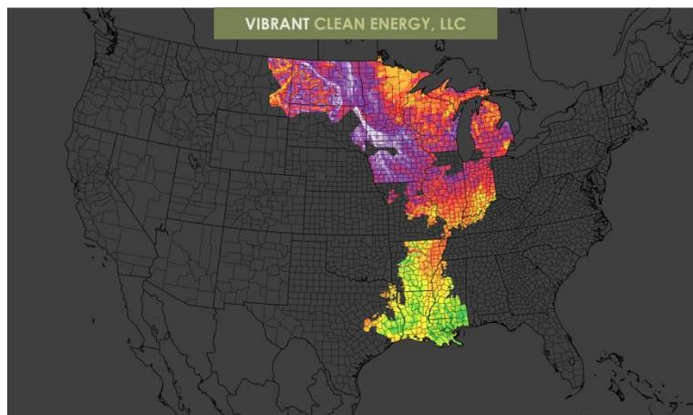
Figure 1: The geographic extent of MISO showing the wind capacity factors at 80m AGL. The MISO footprint will be the core focus of the study.
