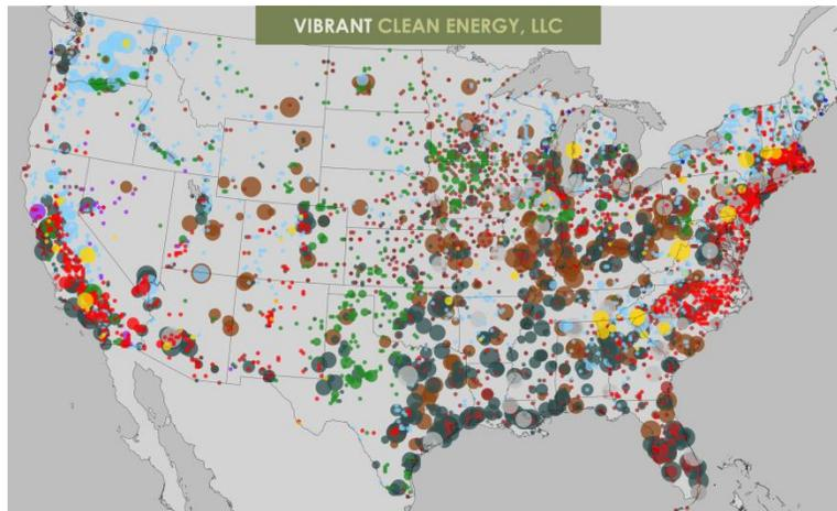
Figure 3: WIS:dom representation of existing (and proposed) Generation across the contiguous United States. Currently there is over 1,100 GW of installed capacity and another 120 GW in queue for construction.
