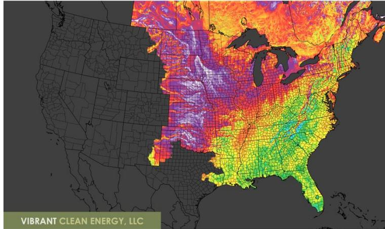
Figure 2: The geographic extent of the Eastern Interconnect and its associated wind capacity factors. The WIS:dom optimization model will represent the whole of the Eastern Interconnect for some sensitivities to determine its impact on MISO siting enhancements.
