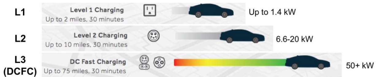
Fig. 4. Comparison of charging speed standards used with EVs. Source: Authors.
