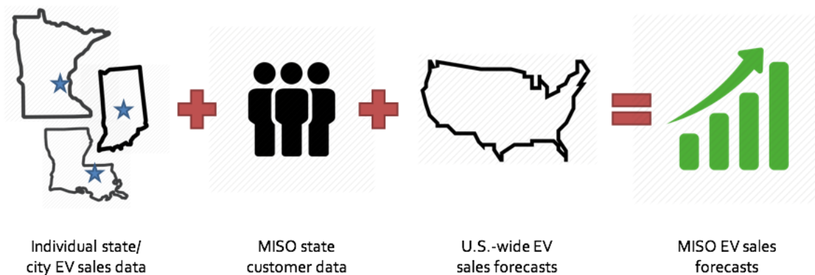
Fig. 8. Schematic of EV forecasting approach used for MISO. Source: Authors.
