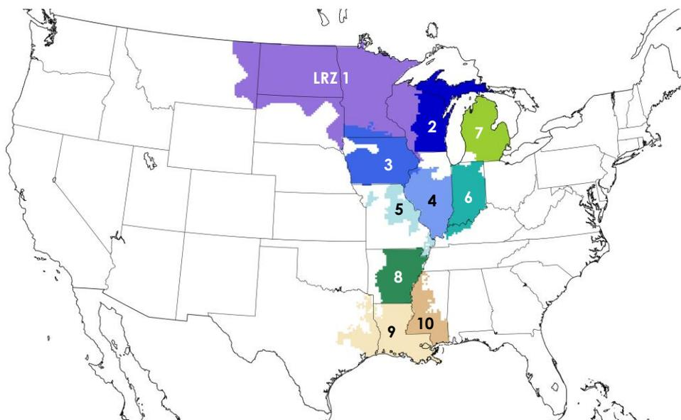
Figure 4: The geographic extent of the present study. Each of the LRZs has a separate color and is labeled. The model balances generation, transmission, and demand within each LRZ. The model does not consider transmission to or from outside MISO.
