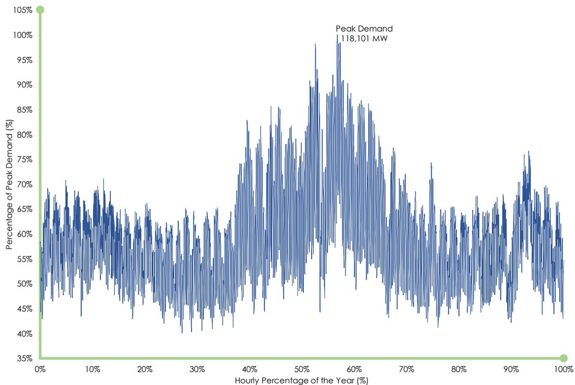
Figure 5: The peak-normalized aggregated demand profile for the entire US MISO footprint. The aggregated demand is the sum of the demand profiles in each of the LRZs. The year chosen as a reference was 2006. The peak demand was 118,101 MW. The demand profiles were time-aligned with the wind and solar power dataset.
