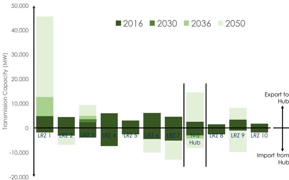
Figure 11: The transmission capacity at each time horizon of the CO RC NCT scenario. The exploitation of higher quality wind resource in LRZ 1 is facilitated by significant transmission capacity. The dark green is the existing transmission capacity. Where lower amounts of wind and solar PV are deployed, transmission expansion is not as critical.
