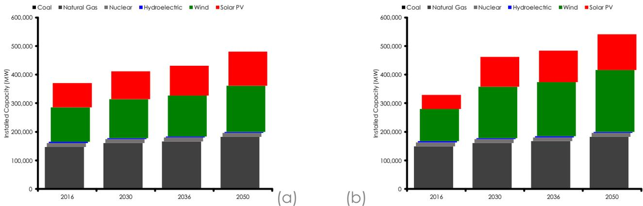
Figure 14: The capacity of generators on the MISO grid for the LMO RC CT (a) and LMO RC NCT (b) scenarios. The expanded transmission facilitates further deployment of wind and solar PV. The transmission does not significantly alter the amount of natural gas developed, although it is slightly decreased.
