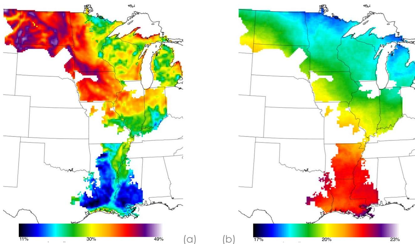
Figure 6: The wind (a) and solar PV (b) average resource for 2006. The average resource is defined as the annual capacity factor. It is clear from the panels that the best wind resources (in terms of capacity factors) are in the north and the best solar PV resources are in the south.
