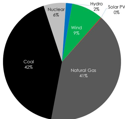
Figure 7: The share of estimated installed capacity on the MISO electric grid in August 2015. The chart shows the share of 223,648 MW of capacity available to the co-optimization procedure at its initialization; where costs are already sunk.
