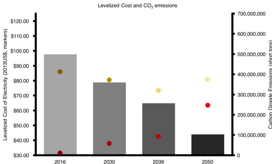
Figure 2: The levelized cost of electricity (LCOE) and the total carbon emissions from electricity production within the MISO footprint. The bars represent the CO<sub>2</sub> emissions (right axis). The red dots symbolize the LCOE when not considering the capital costs of existing generators on the MISO grid, while the yellow dots show the LCOE that includes these capital costs. The scenario is the same as in Figure 1.
