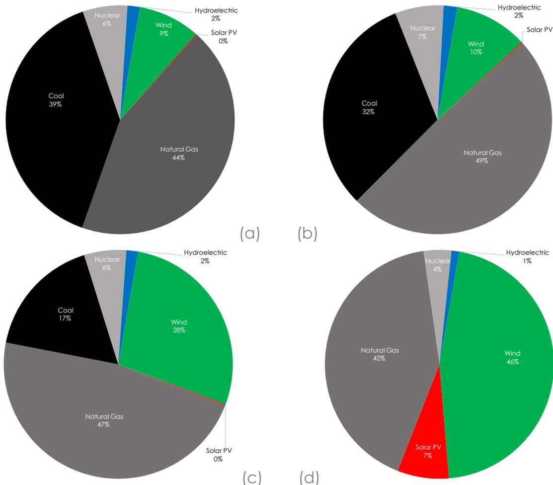
Figure 8: The share of capacity for the four time horizons for the CO RC NCT scenario; (a) 2016, (b) 2030, (c) 2036, (d) 2050. By 2050, with an 80% CO<sub>2</sub> reduction, most electricity comes from wind and solar PV.
