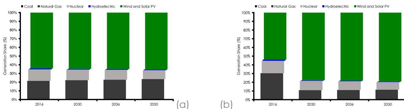
Figure 15: The generation share by technology for the LMO RC CT (a) and LMO RC NCT (b) scenarios. Panel (b) clearly shows the effect of transmission expansion in 2030, when the wind and solar PV generation jumps from ~50% to ~80%. In panel (a), the generation share remains fairly constant, but as the demand is growing, new generators are added to provide the generation in the same proportions between fossil fuel (natural gas) and variable generation (wind and solar PV).
