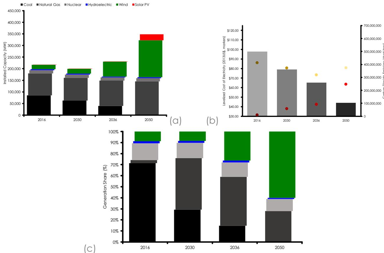
Figure 9: The overall features of the CO RC NCT scenario. (a) The capacity stack for each time horizon, (b) the levelized cost of electricity and carbon dioxide emissions, (c) the generation share by technology (green is wind and solar PV combined).
