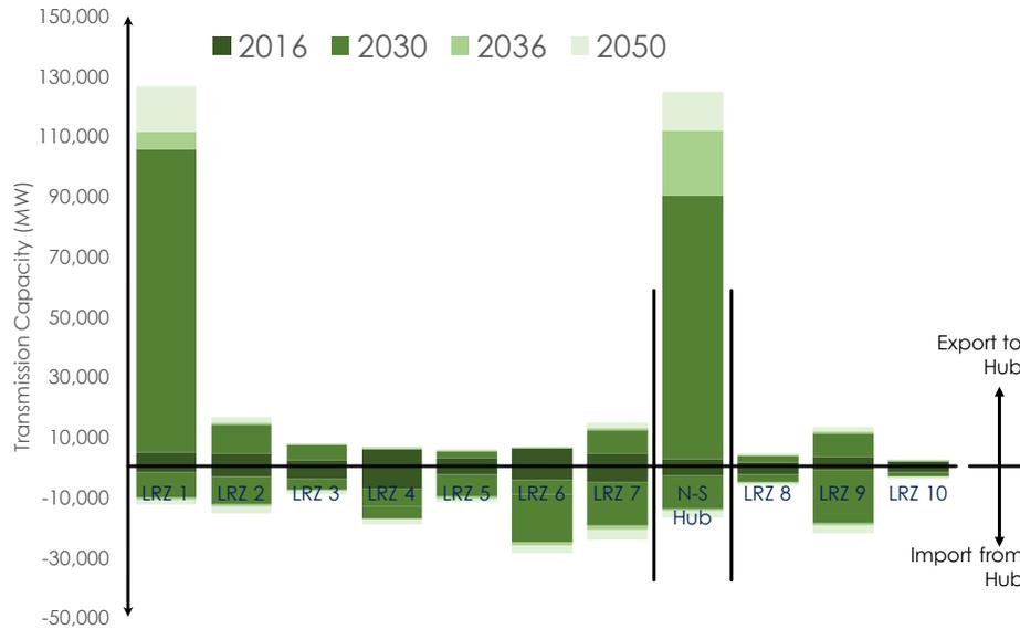
Figure 13: The transmission capacity at each time horizon of the LMO RC NCT scenario. The dramatic exploitation of higher quality wind resource in LRZ 1 is facilitated by significant transmission capacity. The dark green is the existing transmission capacity. The trend is the same as in Fig. 11 for the CO RC NCT scenario, but here it is extended much further.
