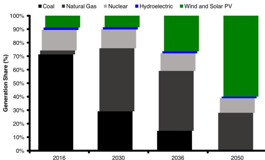
Figure 1: The share of generation for the most dominant sources within the MISO footprint over the four study time horizons. Carbon dioxide emissions are not constrained in 2016, are reduced by 30% by 2030, 50% by 2036 and by 80% by 2050. Transmission expansion is allowed in this co-optimized scenario. By 2050, over 60% of the electricity can be produced by weather-driven renewable sources.
